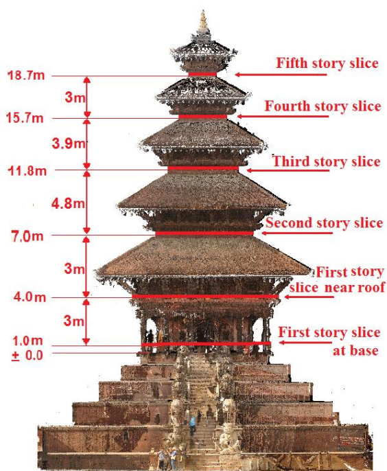
Figure 4.3: Elevation view highlight location of the point cloud slices for floor sections.
